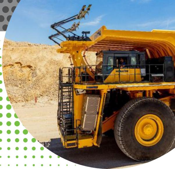
1. Trolley-assist systems utilize external electrical power sources during uphill segments to produce the energy required to power electric wheel motors
