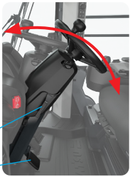
Steering telescopic lock lever Steering tilt lock release pedal
